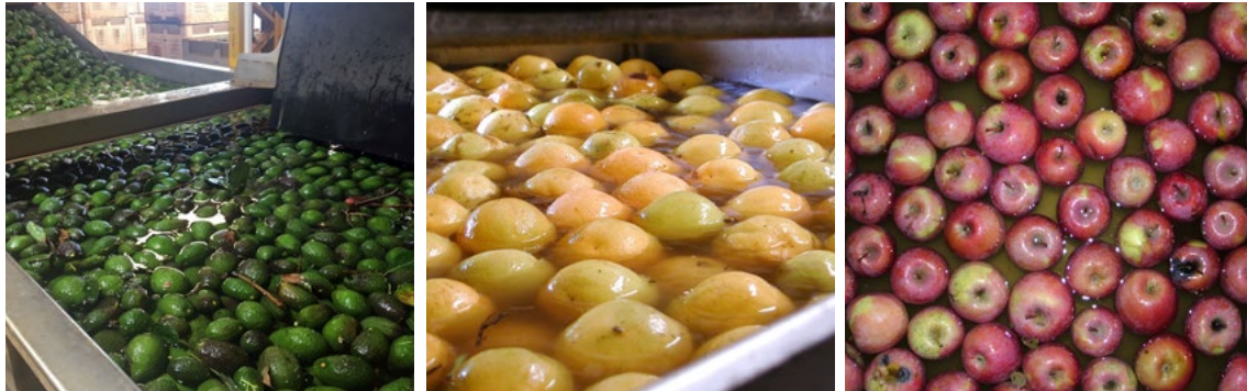
Figure 19. Wet dumps and water flumes are commonly used to transport produce during packing, but can be a significant source of risk if not properly sanitised
