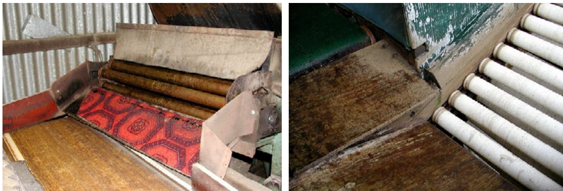
Figure 30. Packing lines should not use absorbent materials such as sponge and carpet, as these cannot be properly sanitised, wood is difficult to clean and flaking paint introduces a potential hazard
