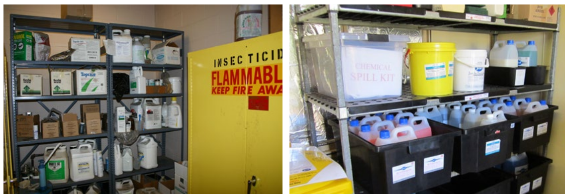
Figure 25. A good chemical store is structurally sound, secure, and has chemicals well organised and in their original containers (left, P McMahon). Flammable items and cleaning products should be kept separately from other chemicals (right, NSW FA)
