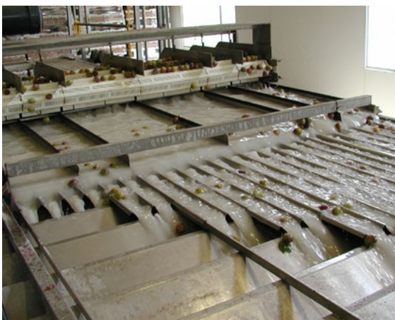
Figure 21. Water containing <1 cfu/100ml should be used to apply fungicides and waxes
