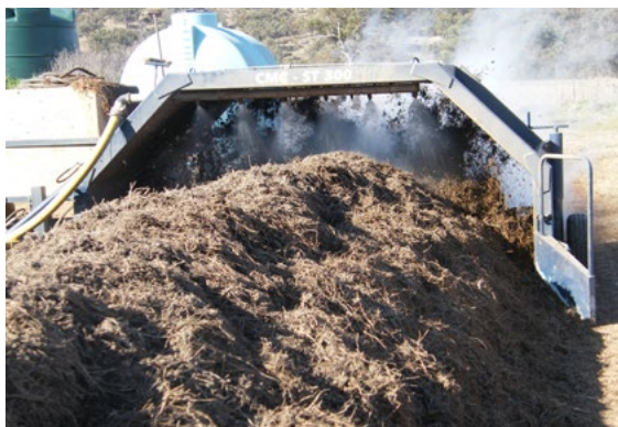
Figure 12. Turning a windrow (left) and an in-vessel static composting system (right) (Global Composting Solutions)
