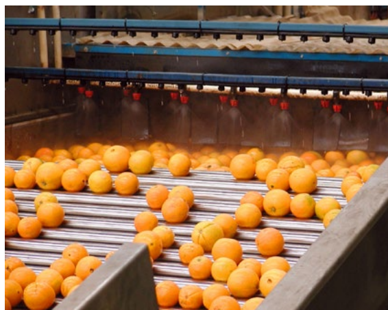
Figure 21. Water containing <1 cfu/100ml should be used to apply fungicides and waxes
