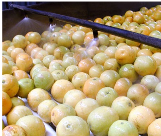
Figure 26. Waxes should be appropriate for the destination market e.g. morpholine based waxes are not approved in Europe
