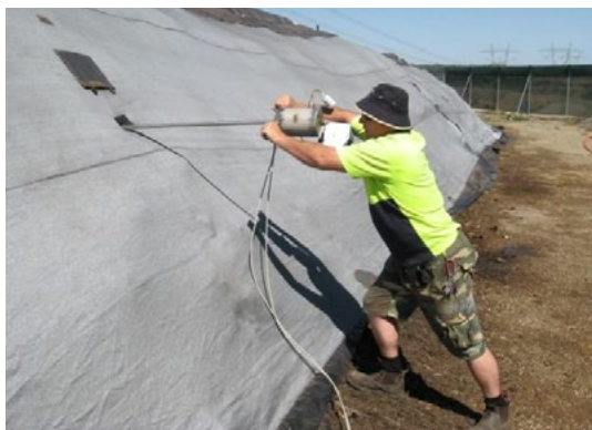
Figure 14. Measuring temperature inside a compost windrow
